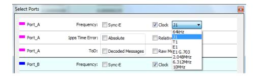
By selecting the desired rate from the drop-down menu for a chosen measurement port, you can now additionaly choose to measure wander for J1 signals, 64kHz frequency (64k + 8k and 64 + 8 + 400Hz formats are also supported by this selection) and 6312kHz frequency.
